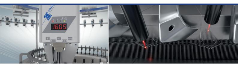
Missing needles can be masked out e.g. when working with cutting line or when producing patterns. To avoid false stops, the number of revolutions before stopping the machine is adjustable.
