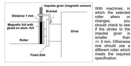
Next, the magnetic foil supplied, must be attached to the levelling roller. As the foil is glued in place, please make sure that the surface to which it is to be fixed to, is absolutely free from any oil or grease.
