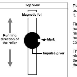
Please apply the foil to the roller using pressure, but do not stretch
