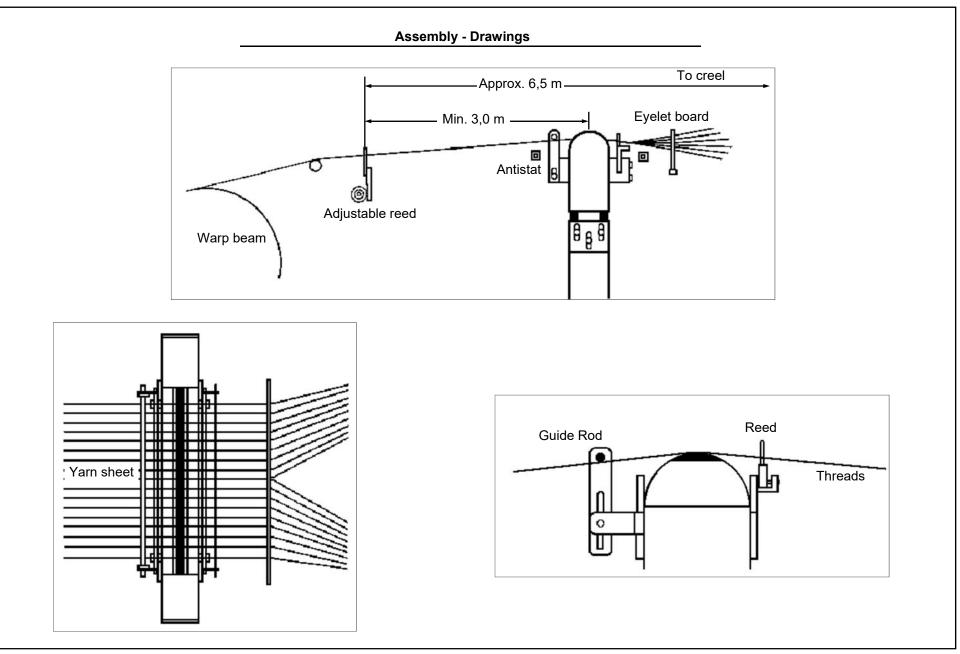
As you will see from the drawing above, to obtain the best possible performance from the yarn inspector, the distance between the warping machine and the creel should be at least 6,5 meters.
