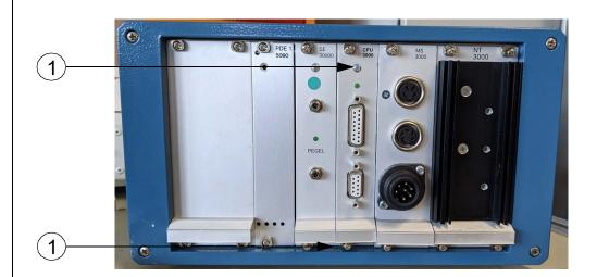
To remove the CPU, the two screws (1) must be unscrewed with a Phillips screwdriver. Then pull out the CPU.
