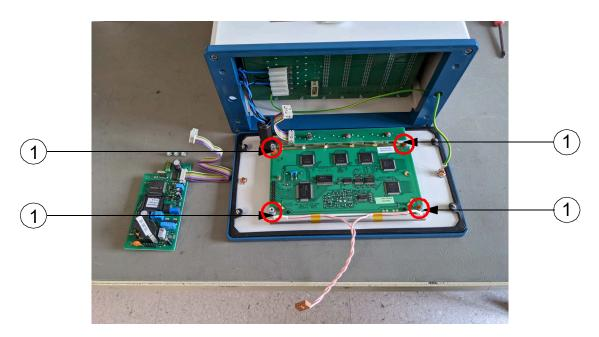
Unscrew the four nuts (1) to remove the display from the front unit.
