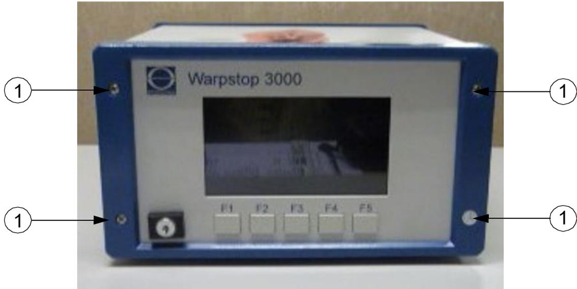
To be able to replace the display, the front unit must be dismounted. To do this, unscrew the four screws (1) with a Phillips screwdriver. The front unit then can be removed.
