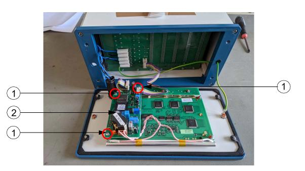
Place the LCD control module (2) on the three stud bolts (1) and fasten the module with the three screws (1)
