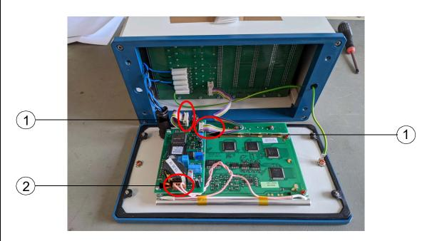
Then the two ribbon cables (1) and the lighting connector (2) must be reconnected.
