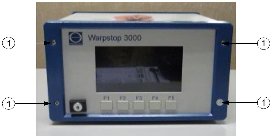
Finally, the front unit is mounted on the control unit again. The front unit is fasten to the control unit with the four screws (1).
