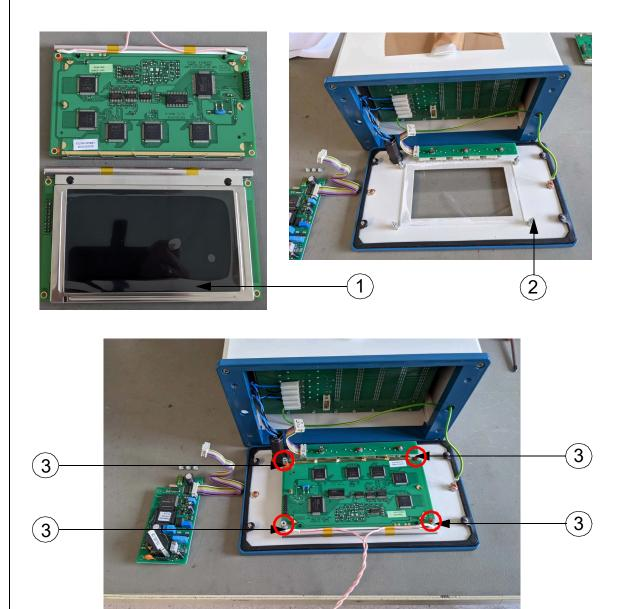
Remove the protective film (1) from the new display.
