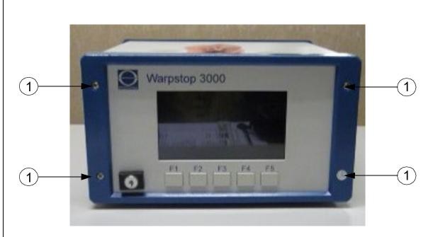
Finally, the front unit is mounted on the control unit again. The front unit is fasten to the control unit with the four screws (1).
