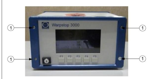
To be able to replace the display, the front unit must be dismounted. To do this, unscrew the four screws (1) with a Phillips screwdriver. The front unit then can be removed.
