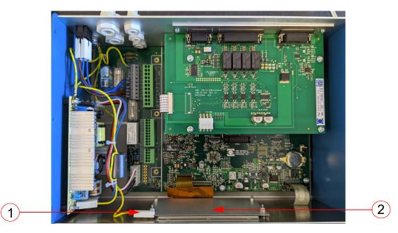
Remove the grounding cable (1) from the display (15121) (2).
