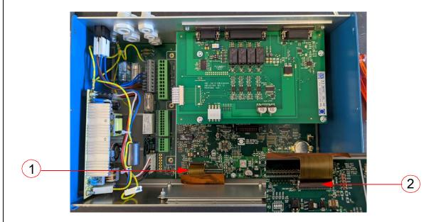
In this step, the flat ribbon cable of the display (15121) (1) must be unplugged. To do this, the locking mechanism of the connector (2) must be opened. Then the flat ribbon cable (1) can be carefully pulled vertically out of the connector (2).
