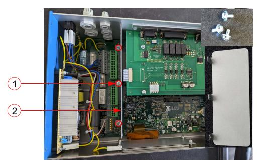
The separation panel housing (2) is then fixed in the control unit with the three screws (13429) (1).
