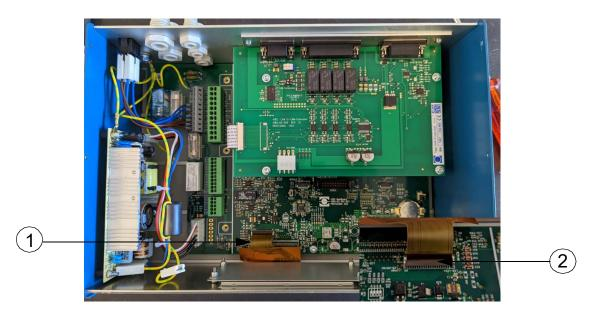
Next, the flat ribbon cabke of the display (15121) (1) must be connected. If necessary, open the locking mechanism of the flat connector. Then the flat ribbon cable (1) can be carefully inserted vertically into the connector (2). The locking mechanism must then be closed.
