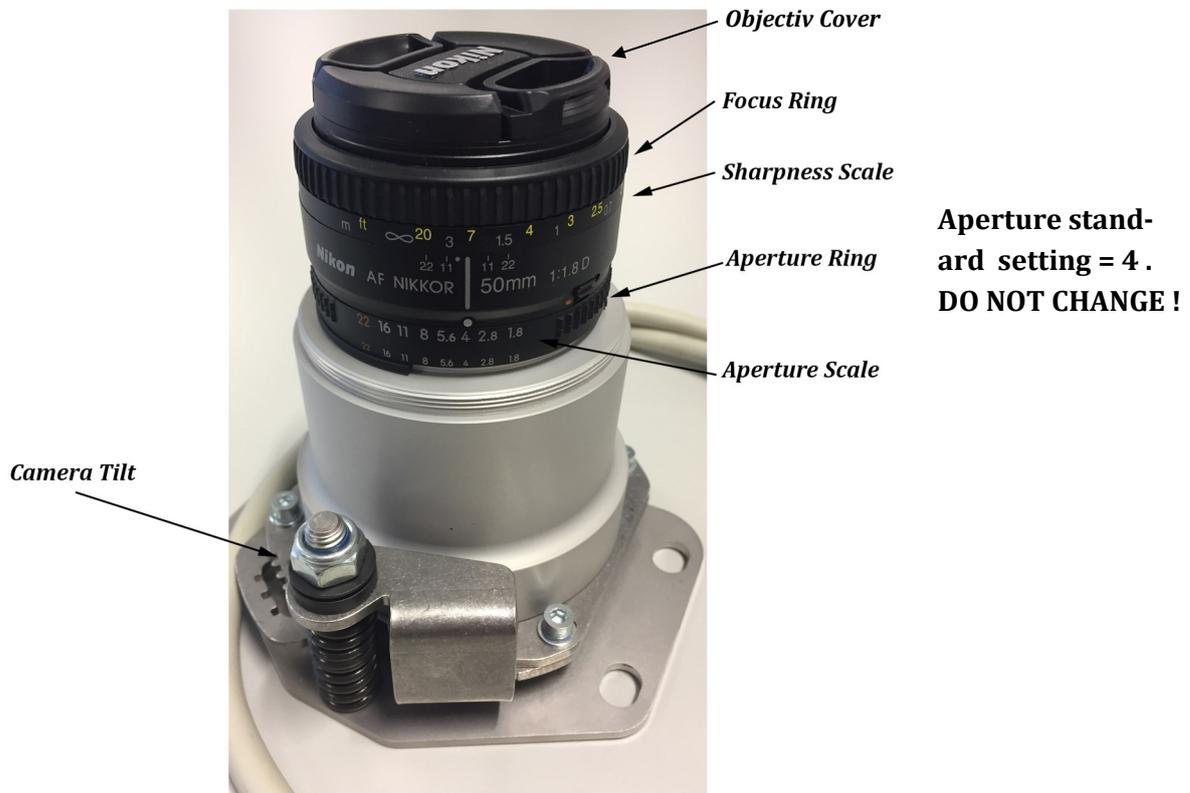
The camera has two adjustment rings and two belonging scales:
